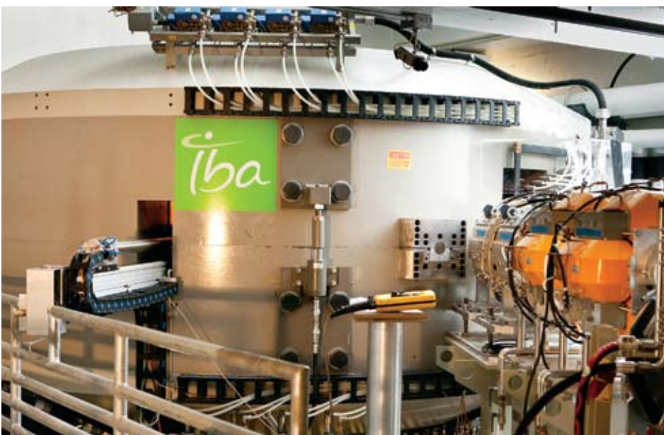
The cyclotron is a particle accelerator that spins protons to two-thirds the speed of light, sending the resulting proton beam through a beam line to 90-ton gantries that sit three stories high. The gantries rotate to allow the beam to be delivered at any angle around the patient.
